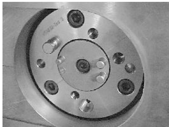
Second bending head developed for CFM 2D forming and welding machine.
