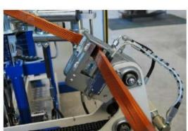
Equipped with hydraulic cylinders for retaining the copper bar with the possibility of varying the locking position depending on the section of the coil that has to be formed.
