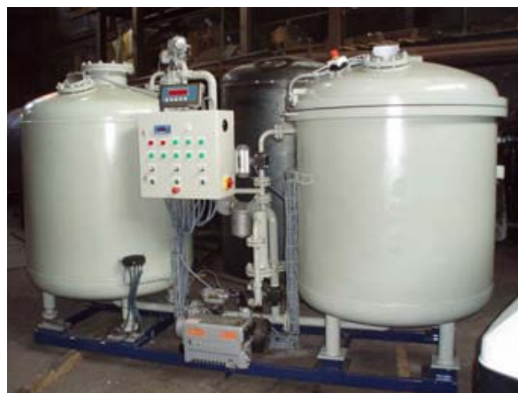
Pre-assembled monoblock VPI system above
