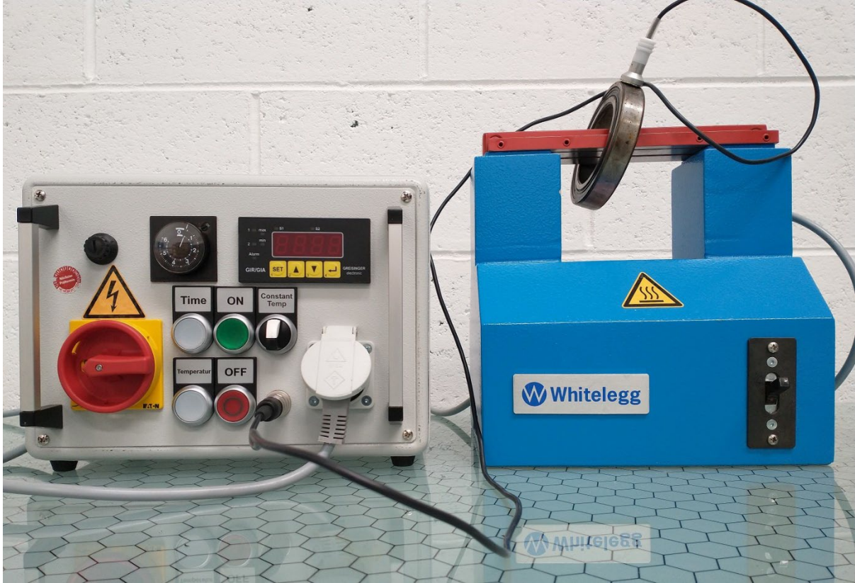
Photo shows IBH-1 with timer, temperature sensor and demagnetisation
